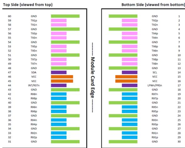
The Active Optical Cable (AOC) pin assignment is SFF-8679 compliant.
